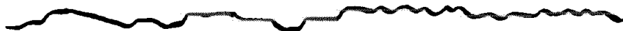
Surface of S. A. E. 1030 Steel, Carburized, Heat-treated and Shot-Peened Magnification 100 Times
