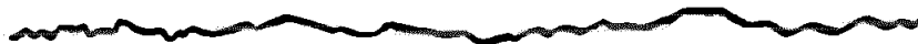
Surface of S. A. E. 1030 Steel, Carburized and Heat-treated but NOT Shot-Peened Magnification 100 Times
