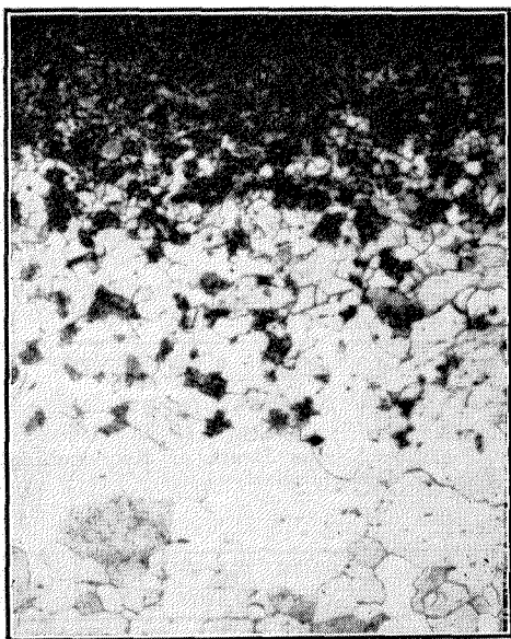
Fig. 6—Photomicrograph Taken Perpendicular to the Surface of a Carburized Test Strip Shot-Peened 5 Minutes at 90-psi Air Pressure. \times 100 . 3% nital etch.
