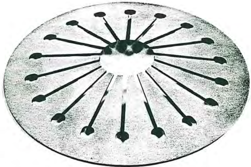
Fig. 3 — Shot peened Belleville spring. Life of this spring and of many other parts is increased by production shot peening.
