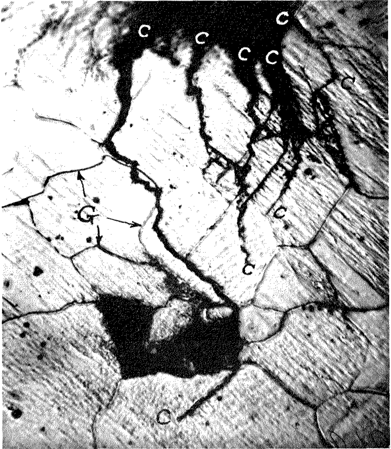
Fig. 4—Photomicrograph of Fatigue Cracks Initiating from Small Corrosion Pit in Low Carbon Steel.
