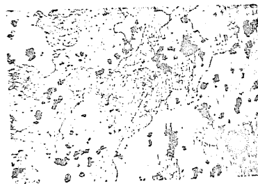
Figure 5. Microstructure of Aluminum 76S-T6 Kellers Etch (250X)
