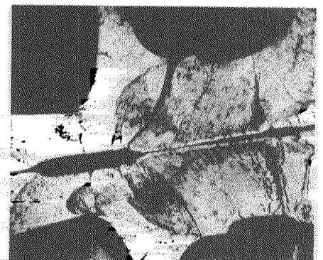
Figure 2—Opposing fracture faces of the corroded aluminum forging.
