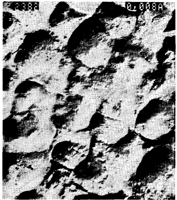
FIGURE 59- 4340 STEEL VAR 48/50 HRC AT 0.0080A AT 200X, PSEF AND TOOL MARKS PRESENT
