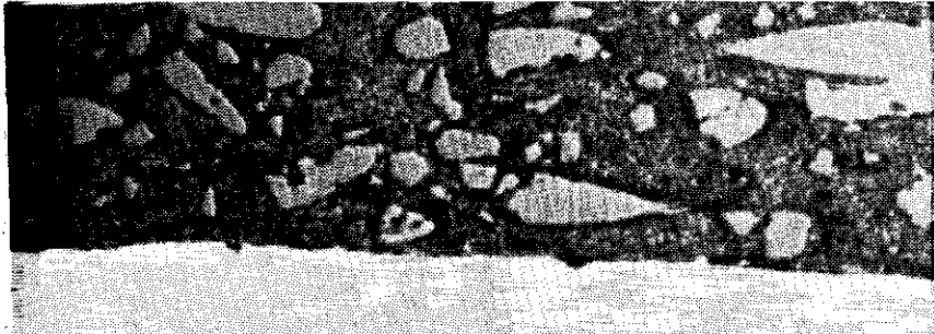
FIGURE 100- 4340 STEEL VAR 48/50 HRC AT 0.0020A AT 700X, 25% BROKEN PARTICLE CONTENT IN MEDIA, NOTICE ACCICULAR IMPINGEMENTS AND EROSION
