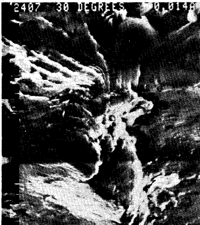
FIGURE 24- 7075-T73 ALUM AT 0.0140A FIGURE 22 AT 1000X - PSEF
