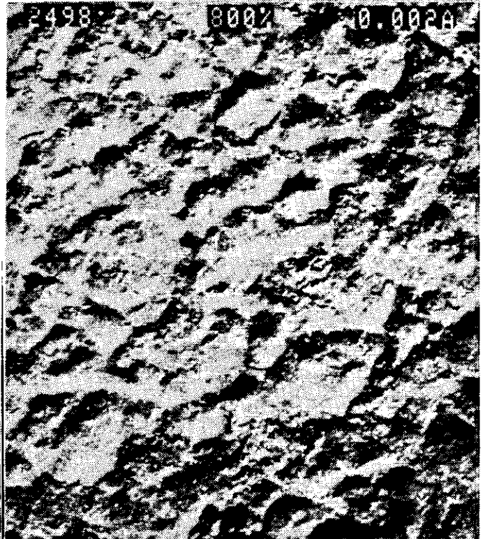
FIGURE 76- 7075-T73 ALUM AT 0.0020A AT 800% AT 200X, IMPINGEMENT PERIPHERY BEATEN DOWN
