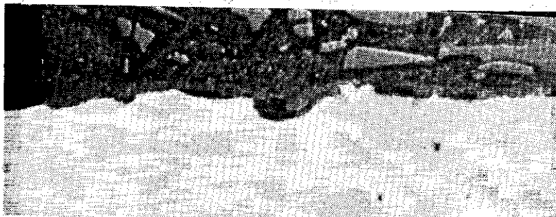
FIGURE 92- 7075-T73 AT 0.0020A AT 700X, WITH 25% BROKEN PARTICLE CONTENT IN MEDIA, NOTICE ACCICULAR IMPINGEMENTS
