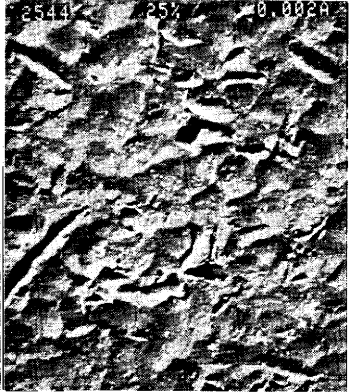
FIGURE 89- 7075-T73 ALUM AT 0.0020A, 25% BROKEN PARTICLE CONTENT, ACCICULAR IMPINGEMENT, 200X
