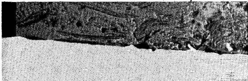
FIGURE 121- 4340 STEEL VAR 48/50 HRC, 0.0020A AT 60 DEGREE ANGLE OF IMPACT, NOTICE "WAVE" CRESTING IN DIRECTION OF MEDIA IMPACT ANGLE (FROM UPPER RIGHT TO LOWER LEFT AT 60 DEGREES TO SURFACE), 700X
