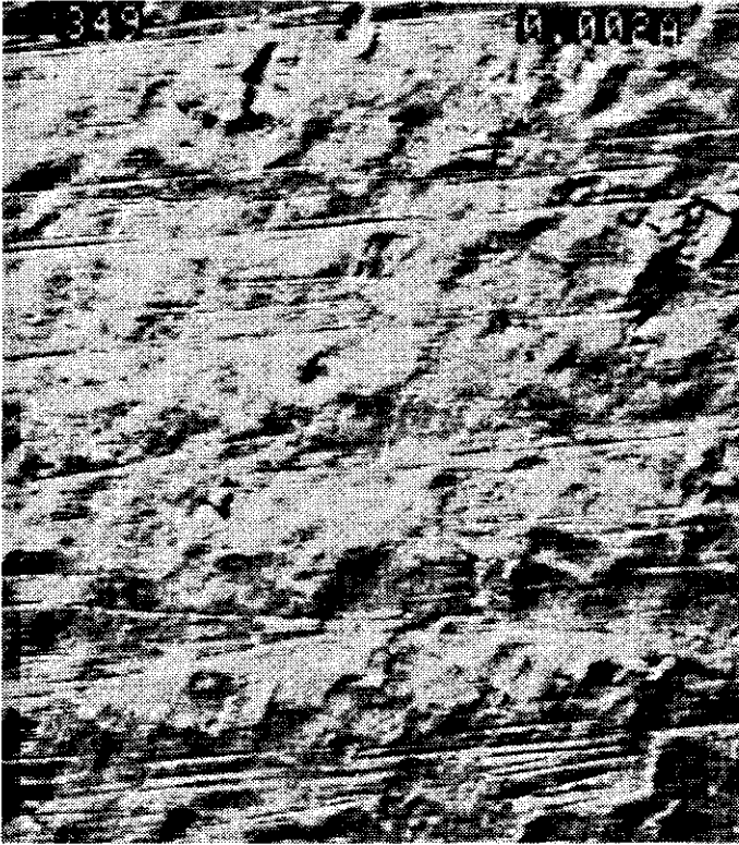
FIGURE 80- 4340 STEEL VAR 48/50 HRC AT 0.0020A AT 200X, 100% WORKPIECE SATURATION, TOOL MARKS VISIBLE
