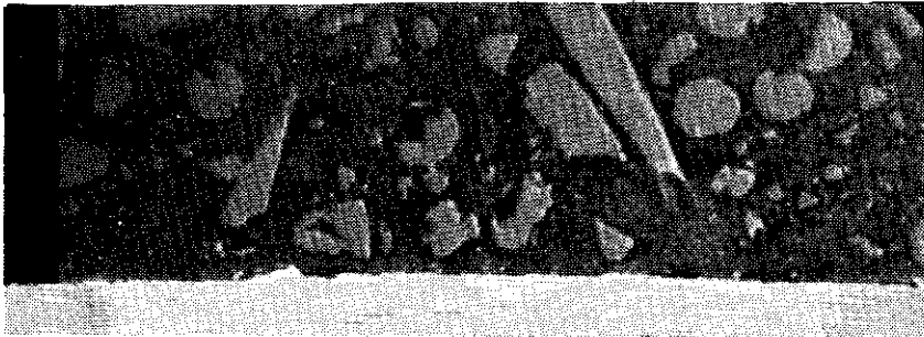
FIGURE 101- 4340 STEEL VAR 48/50 HRC AT 0.0020A AT 700X, 50% BROKEN PARTICLE CONTENT IN MEDIA, EROSION CONTINUES
