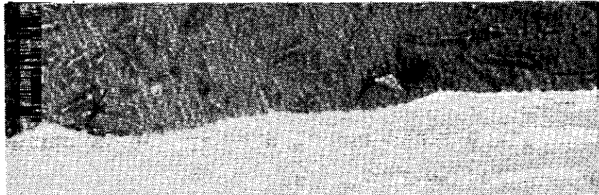
FIGURE 119- 7075-T73 ALUM., 0.0020A AT 60 DEGREE ANGLE OF IMPACT, 700X, NOTICE "WAVE" CRESTING IN DIRECTION OF MEDIA IMPACT ANGLE (FROM UPPER RIGHT TO LOWER LEFT AT 60 DEGREES TO SURFACE)
