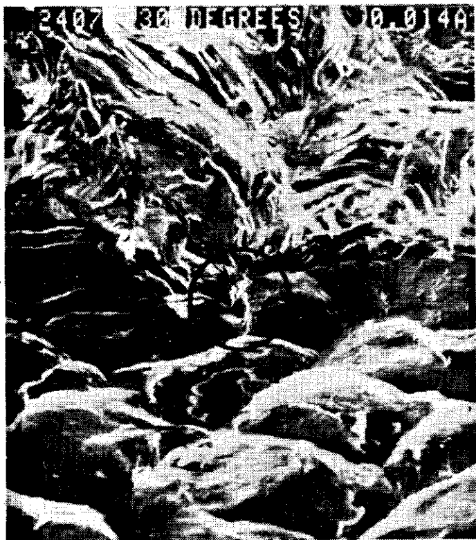
FIGURE 42- 7075-T73 ALUM. AT 0.0140A AT 150X, EXTERNAL INITIATION AT PSEF (ARROW DENOTES CRACK INITIATION SITE)
