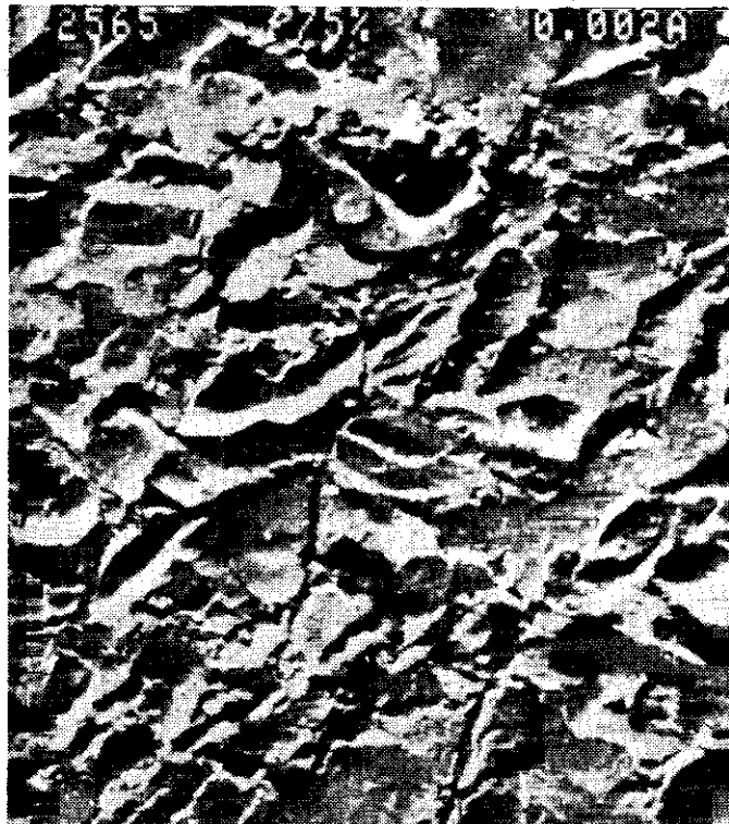
FIGURE 90- 7075-T73 ALUM AT 0.0020A AT 200X 75% BROKEN PARTICLE CONTENT SEVERE ACCICULAR IMPINGEMENTS
