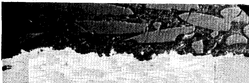
FIGURE 94- 7075-T73 AT 0.0020A AT 700X, WITH 75% BROKEN PARTICLE CONTENT IN MEDIA, SEVERE SURFACE EROSION
