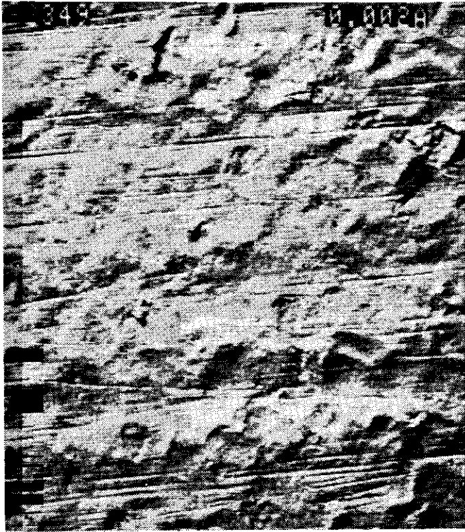
FIGURE 96- 4340 STEEL VAR 48/50 HRC AT 0.0020A, LESS THAN 2% BROKEN PARTICLE CONTENT, 200X
