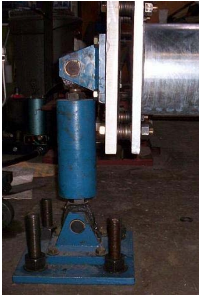
Figure 2.2.3 End Restraint that Allows for Rotation and Translation
