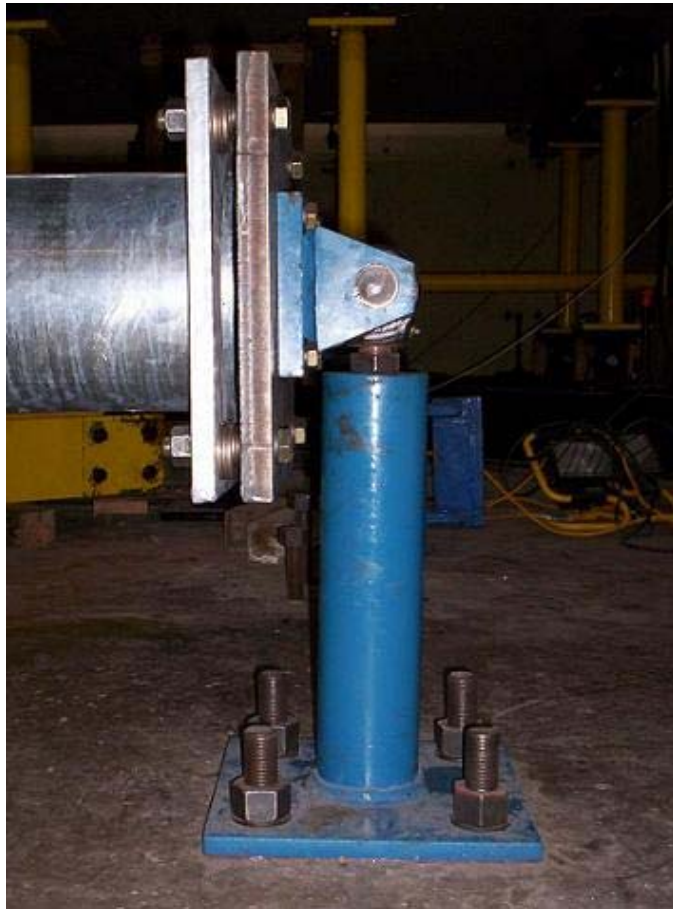
Figure 2.2.2 End Restraint that Allows for Rotation Only
