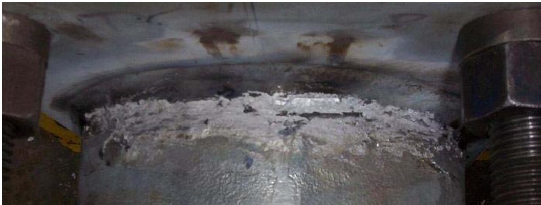
Figure 4.4.3 Mast Arm TXuCLGP After 1 st Controller-Reported Failure (101,865 cycles)
