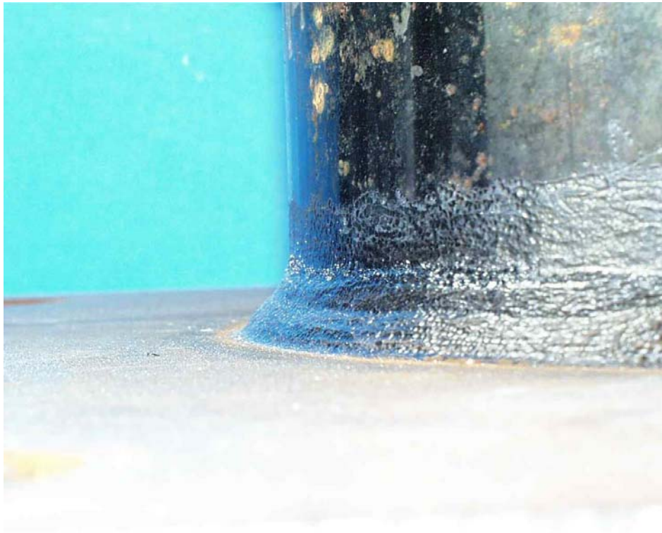
Figure 4.2.1 UIT Application to Both Weld Toes and the HAZ on TXuCLGP
