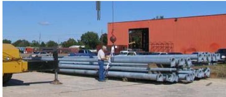
Figure 5.3.1.1 Stockpiled Mast Arms at the TransAmerican Fabrication Yard
