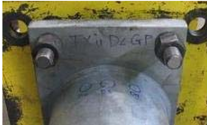
Figure 4.3.3.1 Location of the Middle-Most Temperature Reading Locations (Blue Circles Labeled D2, D3, and D4; The Endmost Temperature Reading Locations are Not Visible in this Picture)
