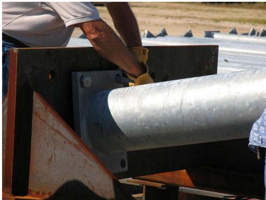
Figure 5.3.1.2 Mast Arm Being Connected to Fixed Testing Stand
