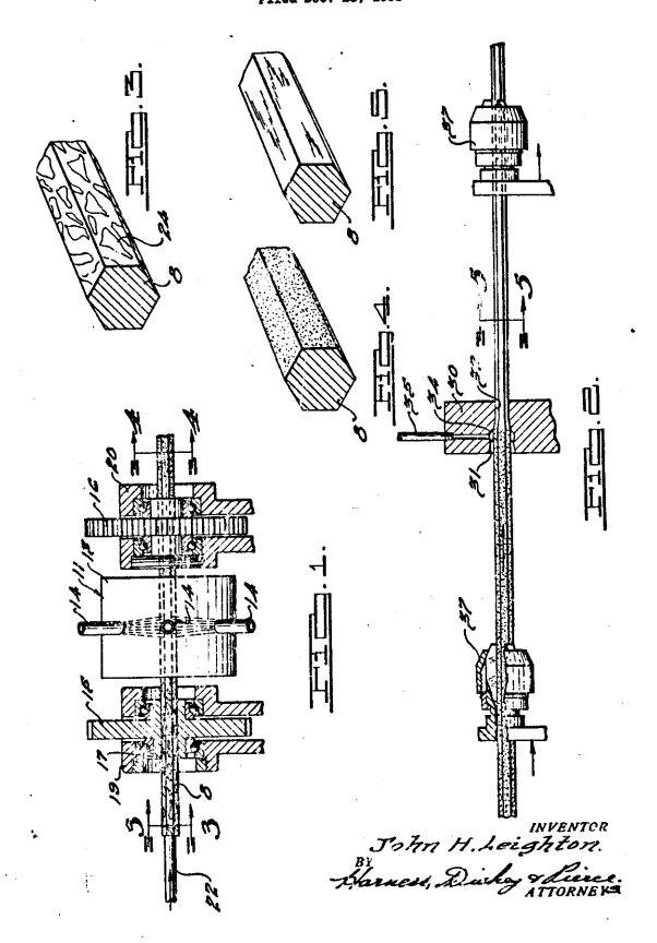
provided for turning the pinions 15 and 16 together and thus rotating the bar, and a push rod 22 has been illustrated as the means for pushing the bar through the pinions and drum although if desired, rollers may be employed for this purpose and such rollers may be disposed at the inlet and discharge side of the apparatus.
