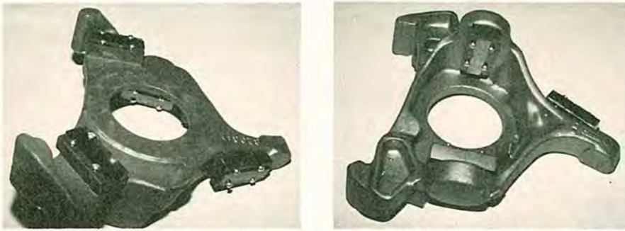
Fig. 6. Side-by-side photos show the front and back views of the steering knuckles used in the test at Wagner Castings. Front view shows the attachment of an Almen block.
