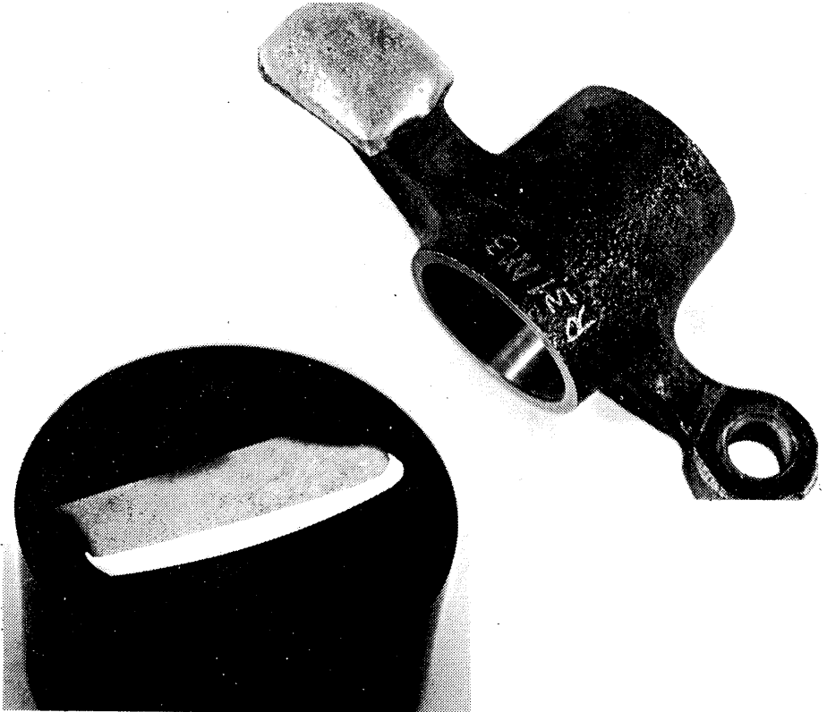
Fig. 19 Rocker-arm after laser cladding and before grinding. Insert metallurgical section of laser clad deposit (white area)
