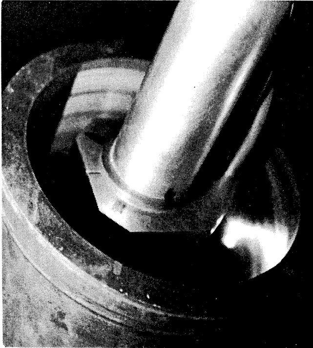
Fig. 7 Seventy percent energy savings are realized during laser hardening of cylinder liners
