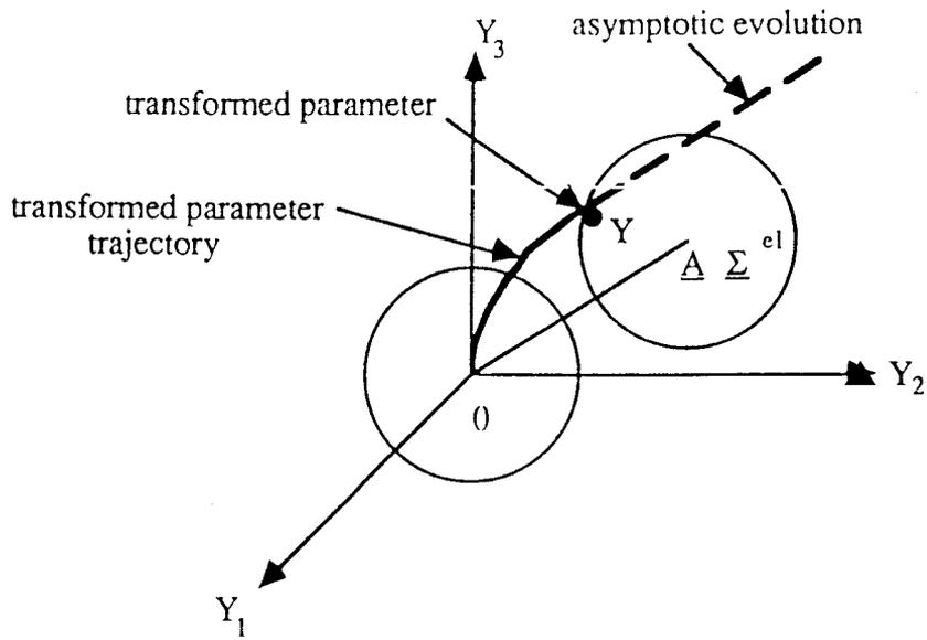
figure 2. Yield surface and transformed parameter evolution.
