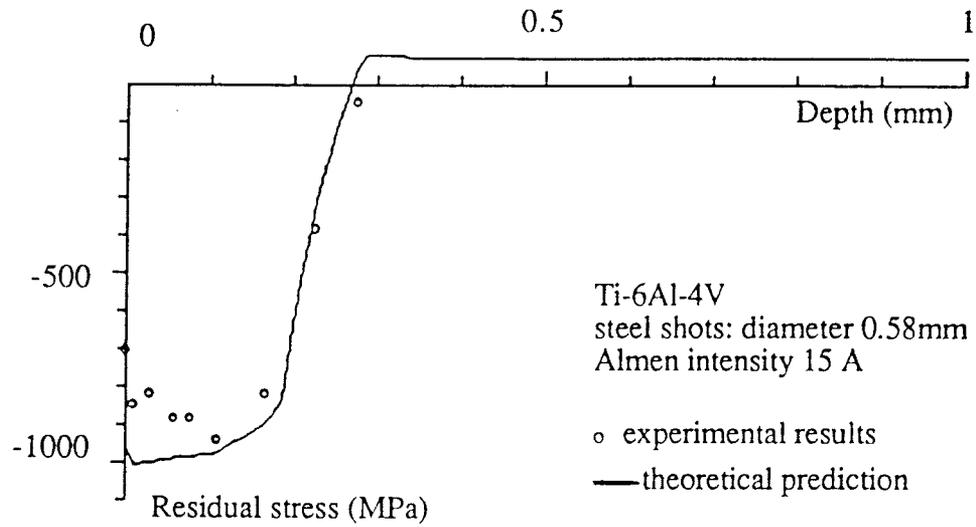
a. Results for titanium alloy Ti-6Al-4V.
