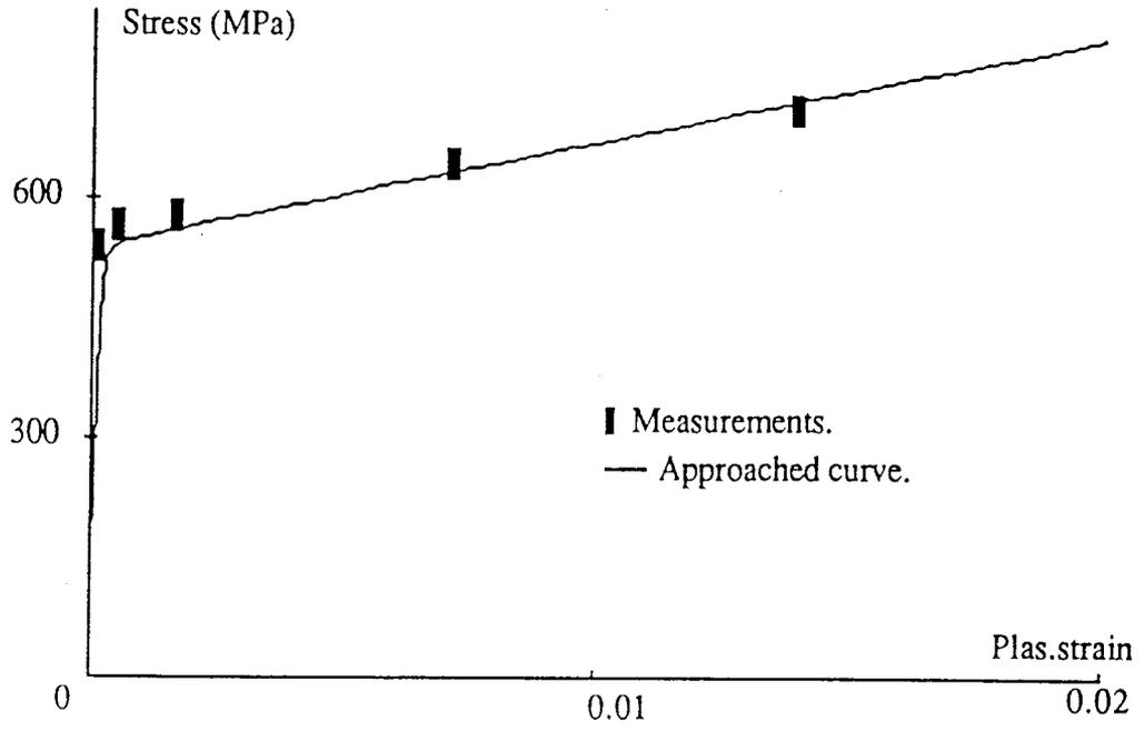
Figure 13. 7075 aluminium alloy behaviour law modelled by a coupled yields block.
