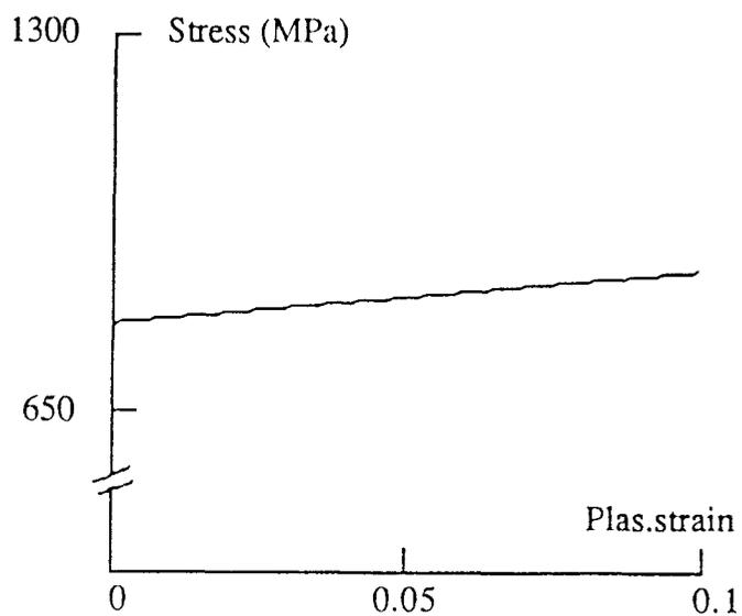
a. Plastic strain-stress curve for a linear kinematic hardening behaviour.
