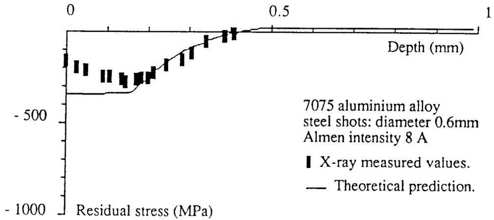
Figure 14. Residual stresses profile introduced in 7075 aluminium alloy.
