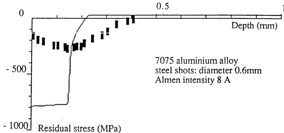
Figure 8. Results for 7075 aluminium alloy
