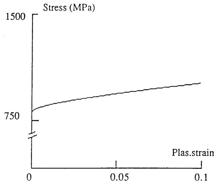
a. Plastic strain-stress curve of a linear kinematic and isotropic hardening behaviour.
