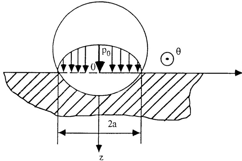
Figure 1. Elastic contact indentation.
