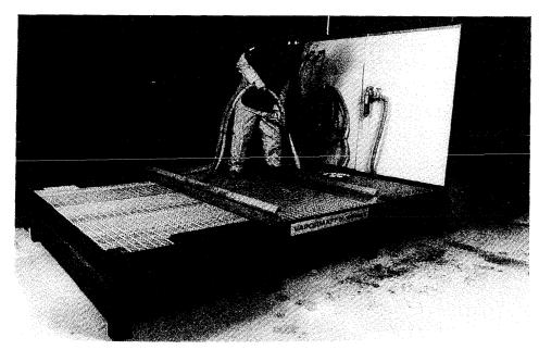
One of the main advantages of the Waterwave System is that it requires no pit or gantry for access as it can sit directly onto the workshop floor and stands only 300 mm. (1') high. A further option can be provided with the same facilities in a booth structure which can be used outside if workshop floor space is at a premium.
