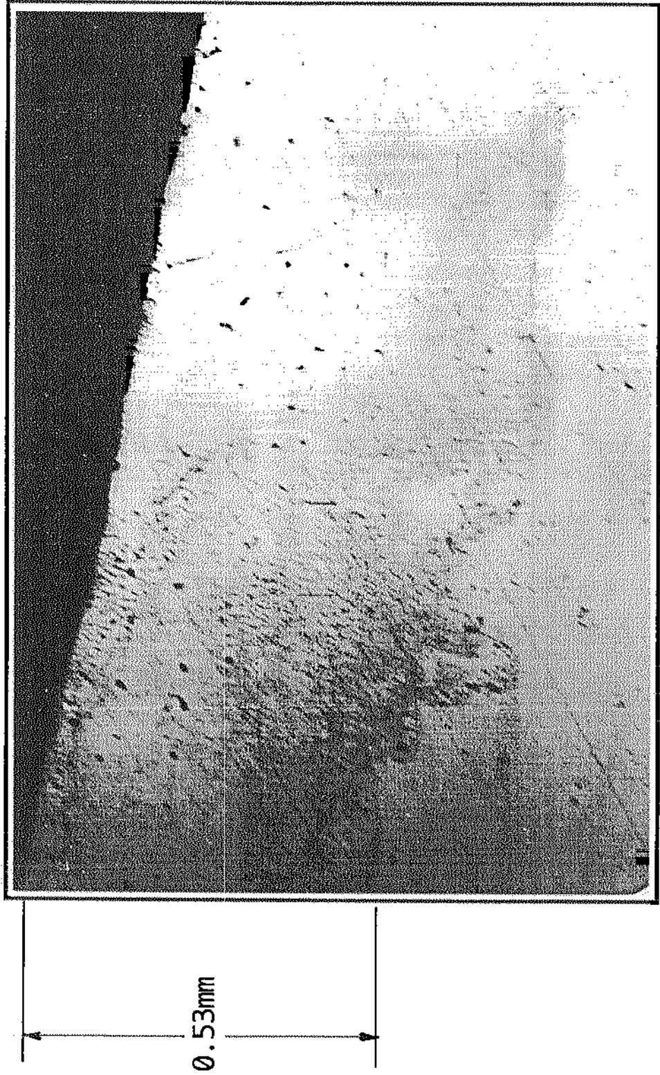
Figure 3.15: Depth of compressive layer after shot peening to an intensity of 10A, and coverage 200% (100X)
