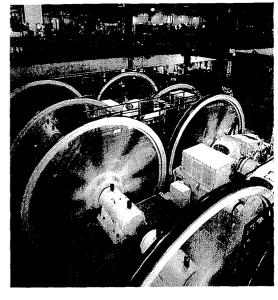
The winding machinery that pulls the 56,000 ft. of ever-moving cable on which San Francisco's cable cars depend for their movement, can be seen in action at the Cable Car Museum.
