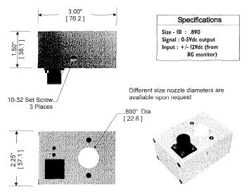
The Sensor is supplied with a 20 ft. cable with a plug in connector on one end and leads on the other, for easy installation. The cable may be cut to length to suite installation.
