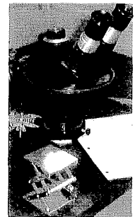
Inspecting shot sample in 1/2 by 1/2 field with 20x magnification
