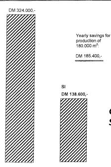
**Operating Cost Comparison** SI Shot-Blasting Plant versus Conventional Plant
