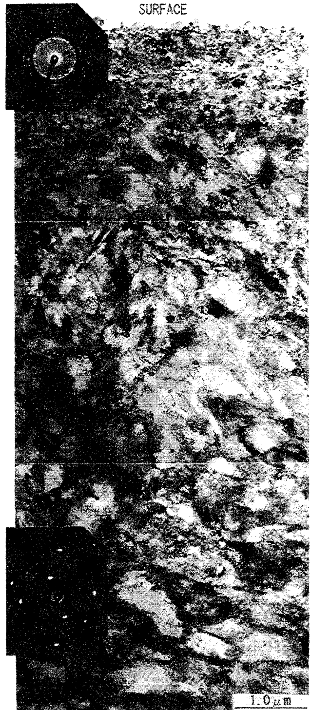
Fig. 8 TEM micrograph and electron diffraction patterns in the as-nitrided high-strength SOTHN wire surface layer
