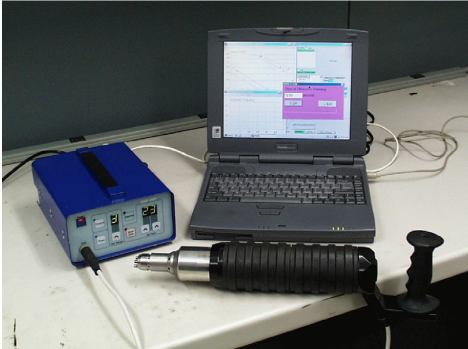
Figure 4. Advanced computerized complex for Ultrasonic Peening of materials, parts and welded elements
