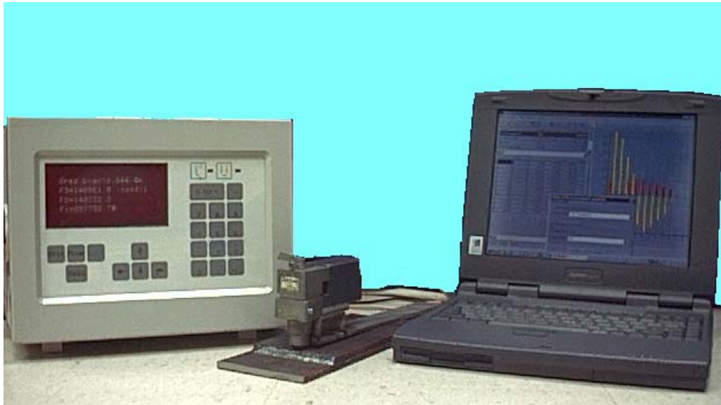
Figure 1. Ultrasonic Computerized Complex for residual and applied stress measurement
