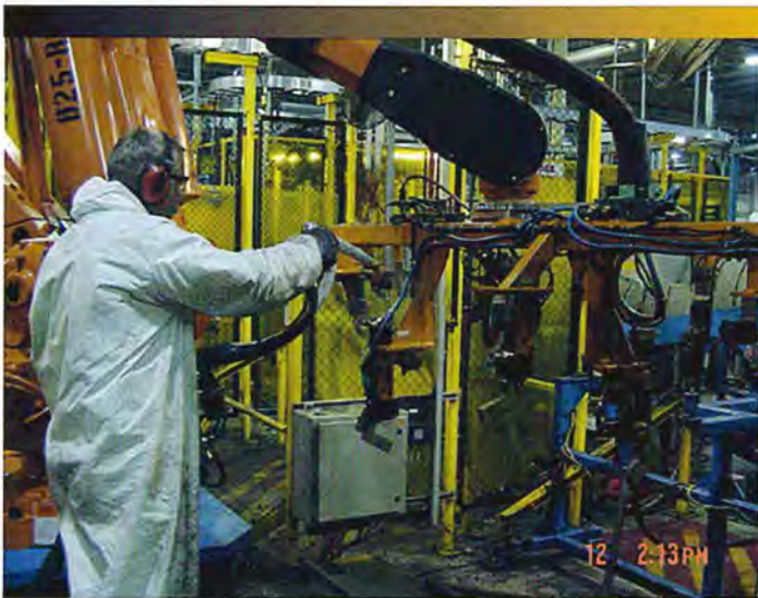
A Wickens technician cleans weld cells, on-site at SKD Milton, with dry ice blasting.
