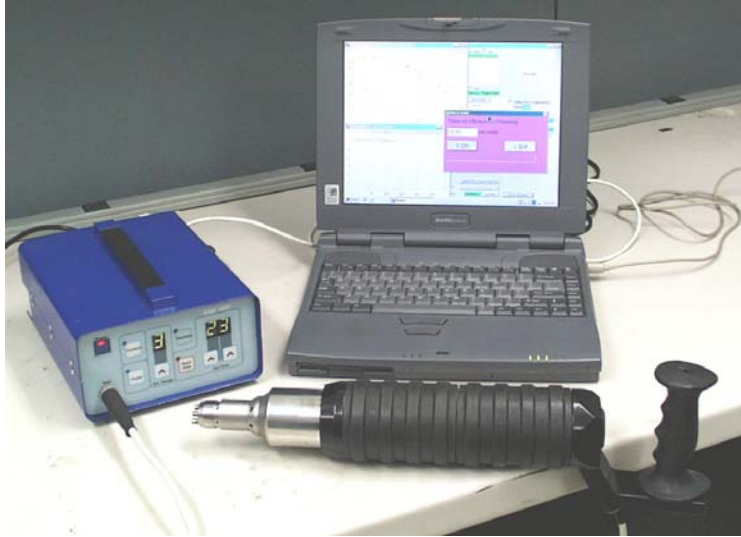
Figure 1. Computerized complex for Ultrasonic Peening of parts and welded elements
