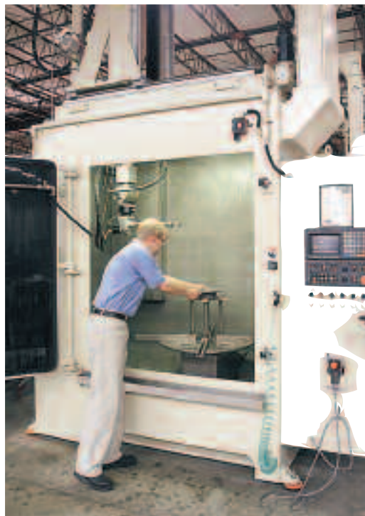
A seal (an aircraft engine part) is being placed on the fixture of a machine at KLM. The UHP waterjet cleaning machine will strip the seal's abrasible coating.
