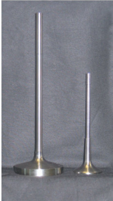
Racecar engines are beginning to employ titanium valves for increased performance due to their light weight, durability, and heat resistance.
