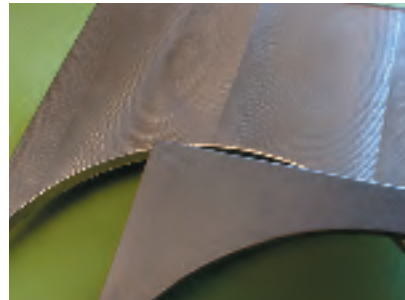
Figure 10. These titanium test coupons show a before and after example of mass finishing processes being used to blend in milling cutter paths. Transforming the positively skewed surface profiles of machined parts into parts with isotropic and negatively skewed surface characteristics can be an important element in any program where surface improvements are being developed to improve wear resistance and metal fatigue resistance on critical parts.
