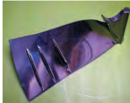
Figure 8. This large power generation turbine blade was made utilizing 6-axis machining technology. Centrifugal barrel finishing technology was used to clear and blend in the milling cutter paths and then develop very refined and burnished isotropic surfaces in the foil area.
