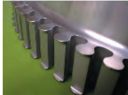
Figure 9. This large aircraft engine turbine disk has been processed with the Turbo-Finish method. This dry abrasive finishing method has been successful in bringing mass media finish economies to large complex rotationally oriented parts while simultaneously developing significant compressive stress. In addition to the uniform and consistent edge contours developed, the method also produces highly sophisticated isotropic surface finishes by radically altering the character of the as-machined or as-ground surface finish. PHOTO courtesy Dr. Michael L. Massarsky, Turbo-Finish Corporation
