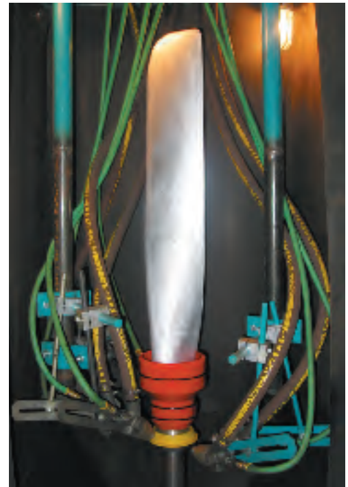
The customer processes various sizes of parts with unique fixtures and masking for each set up.
