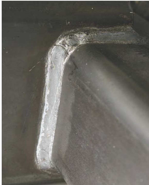
Figure 10. View of welds connecting tubes in as-welded condition (a) and after application of UP (b).
