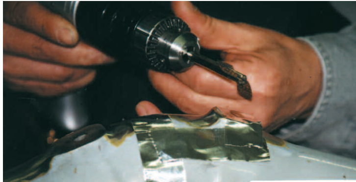
Flapper peening is a manual shot peening process so artisan training is crucial.
