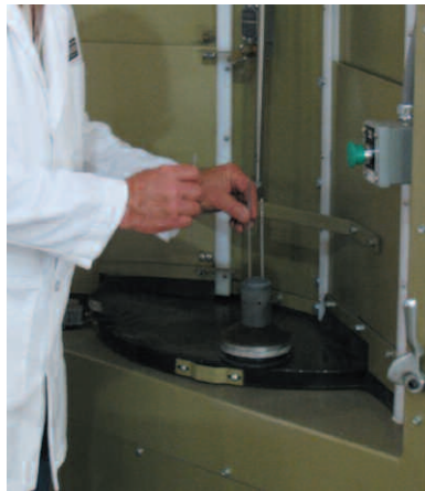
Rigid endoscope components are loaded on a fixture on a ZERO A-200 indexing turntable cabinet
