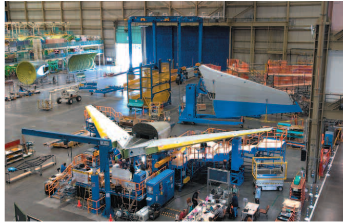
This picture, taken June 13, shows the horizontal stabilizers attached to the tailcone with the vertical fin in the background. Final assembly of the first 787 began on May 21 at the Boeing facility in Everett, Wash. The Dreamliner was scheduled to roll out on July 8, 2007. Image provided by The Boeing Company.
