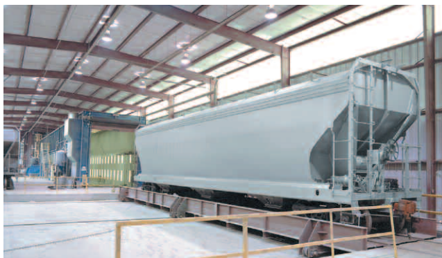
Autoblast and manual touch-up
