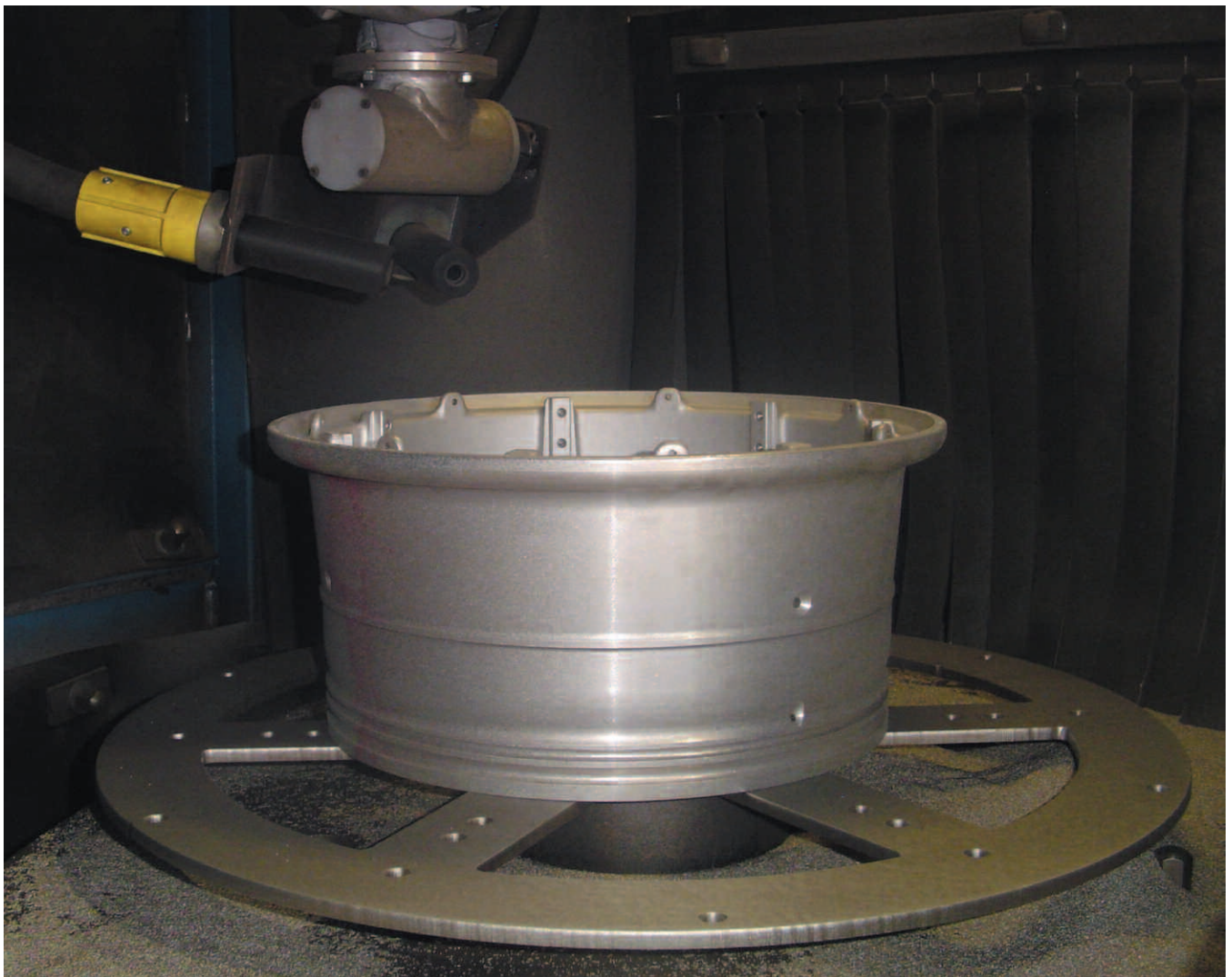
Part touched-up by nozzles after wheelblast
