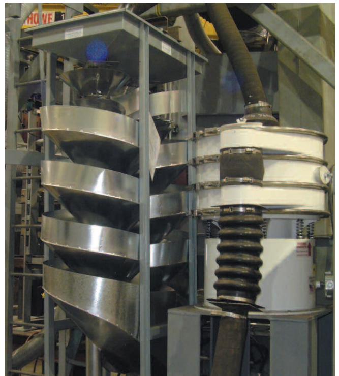
Vibratory Classifier - continuous classification for consistent media size
