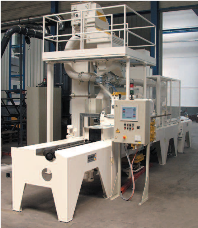
This blasting machine is used to shotpeen stabilizer bars made of manganese steel.
