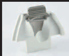
Hand-crafted masters ready for silicone molding
