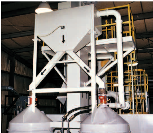
Media bin with MagnaValves. During a blast cycle, 1,530 lbs of shot are used per minute.
