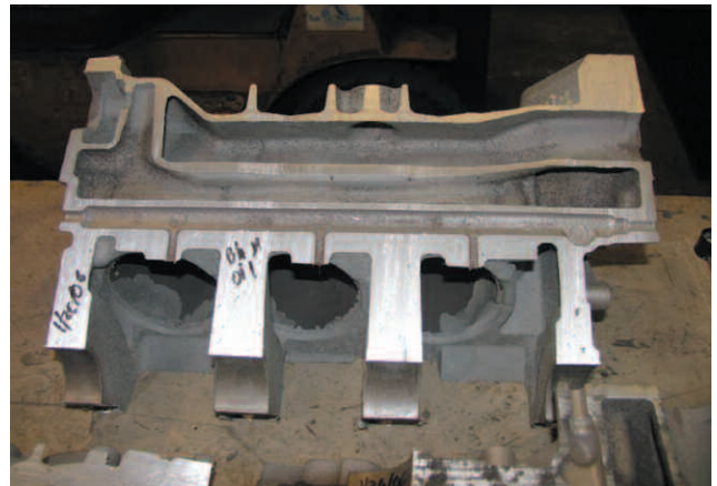
After: A cross-section of an engine block after blast cleaning. The customer specification states that there is to be no more than three grams of sand in the passage after cleaning. Engineered Abrasives' machine removes 100% of the sand from the casting.
