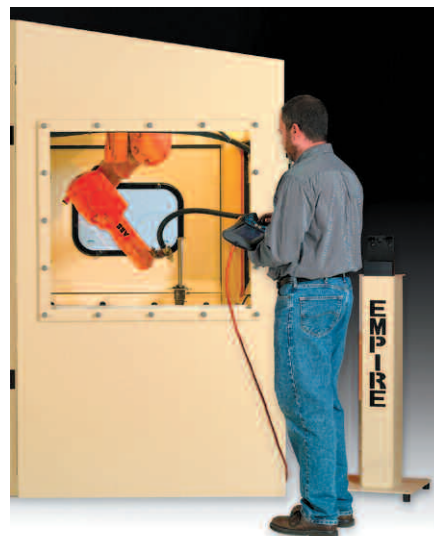
(Fig. 6) Teach pendant provides a fast, flexible means for programming robotic blast machines. Visitors to Empire's test laboratory and demonstration room are encouraged to give it a try.
