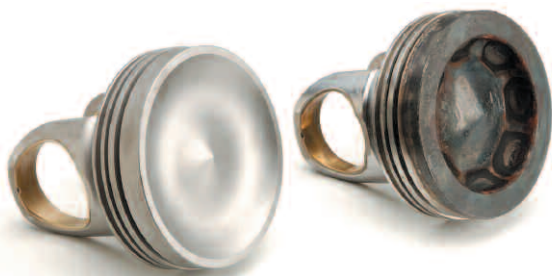
(Fig. 4) Lab work and number crunching found improved tactics for cleaning pistons. Less pressure and more expensive media reduced per-unit costs by 30%.
