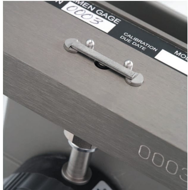
An Almen mini-strip mounted on the gage.
