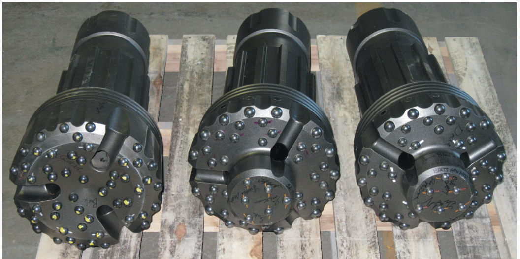
National Peening shot peened these drill bits for Center Rock Inc., a company that used them in their "hole opener" drill to widen the Chilean miner's rescue shaft. Note the signatures of the Center Rock crew.
