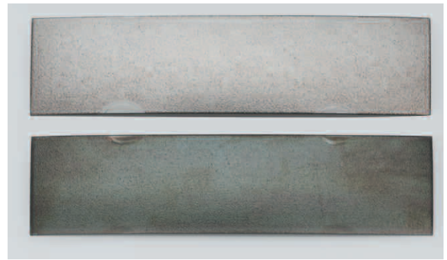
Figure 1. These strips underwent the same peening process. Verification of uniform coverage is easier on the new strip with Coverage Check Finish than on the darker, mottled strip.
