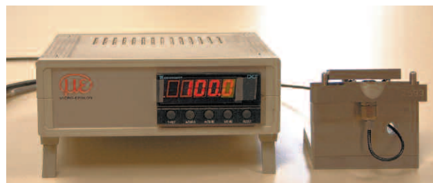
Figure 3. An EI "super" gage with .01000" certified step block. EI has two super gages that measure prebrow to a resolution of 0.00001" and meet SAE J 442 and AMS 2430 for #2 Almen gages. The readings from the gages are continually compared and monitored for accuracy.
