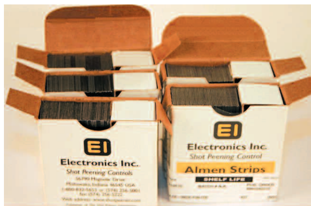
Figure 1. The box on the left holds the newer EI strips and the "earlier" EI strips. The ends of the earlier EI strips are darker due to a different heat treatment.
