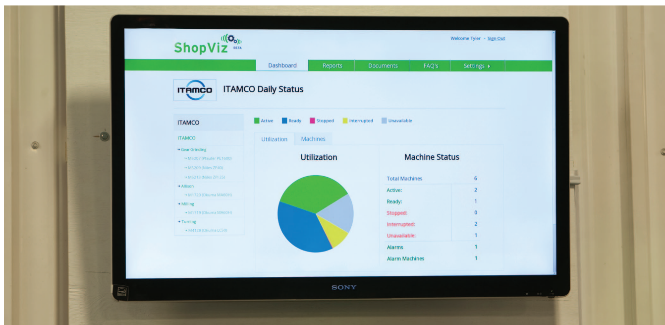
This LCD monitor on a shop wall at ITAMCO displays a dashboard with easy-to-read performance indicators of the gear grinding, milling and turning machines that are connected to its monitoring software. ITAMCO can customize their dashboards to display the performance metrics they want to track.
