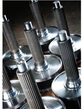
These transmission carriers are ready to be shot peened at ITAMCO.
