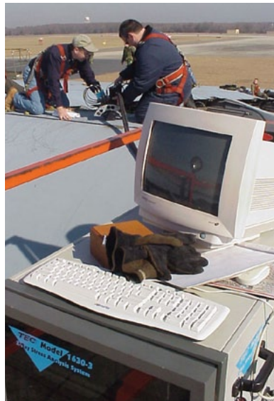
Technicians with Warren-Robbins and TEC are measuring the fuselage on a C-5 transport with a TEC 1630. The computer is recording and analyzing data for rapid and precise results.
