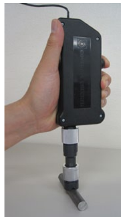
Fig. 9-1) Fix the position of Focus adjustment tool against surface to measure
