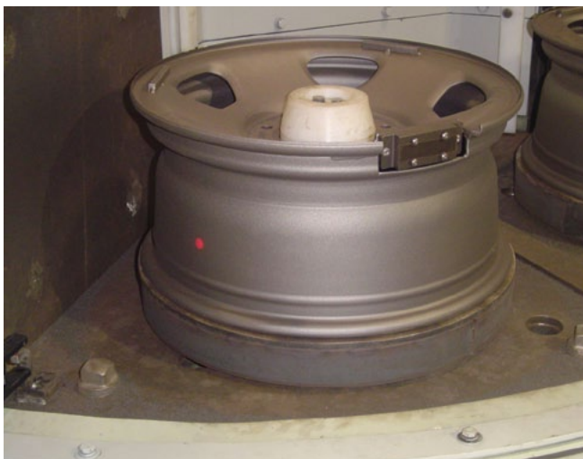
Our customer wanted a shot-peening process to strengthen the welded seam on truck rims.
