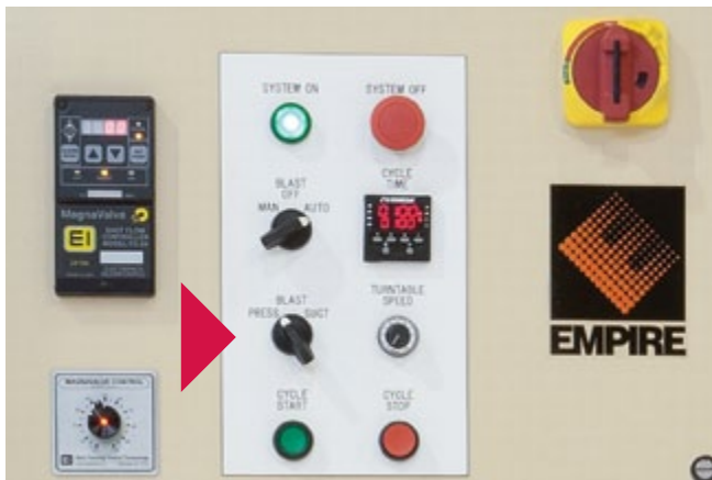
Figure 3. A selector dial for "PRESS" or "SUCTION" on the system's control panel permits the operator to select pressure or suction blasting.
