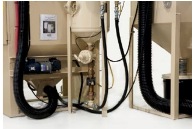
Figure 1. Extended legs supporting the system's 3.5 cubic foot pressure vessel provided sufficient clearance for mounting of a MagnaValve® media flow valve.
