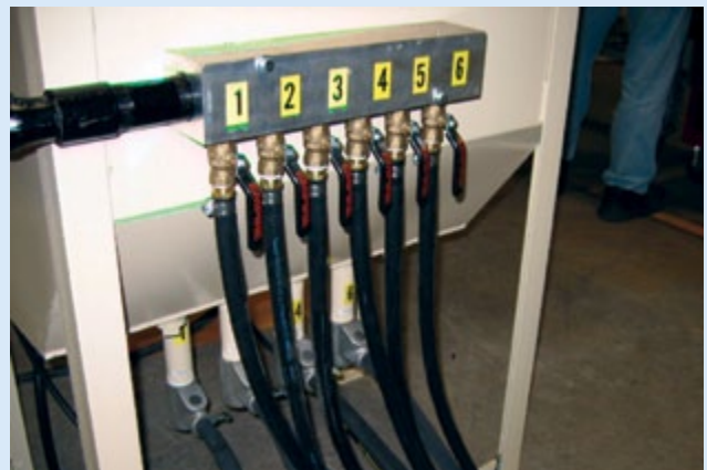
Figure 3. Supplying six blast guns is relatively straightforward as demonstrated by the single air manifold and media hopper, each with six hose outlets.
