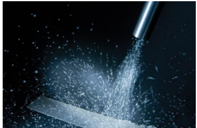
Shot is fired from a blasting gun at a ceramic leaf spring to correct its shape or cause specific warping as desired. (© Fraunhofer IWM, Felicitas Gemetz)
