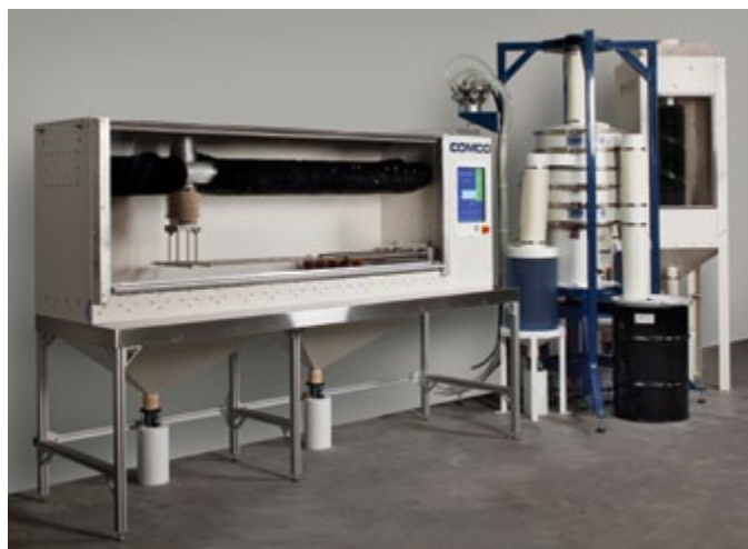
Comco's automated precision shot peening equipment
