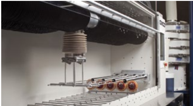
Peening four shafts ID/OD simultaneously for aerospace
