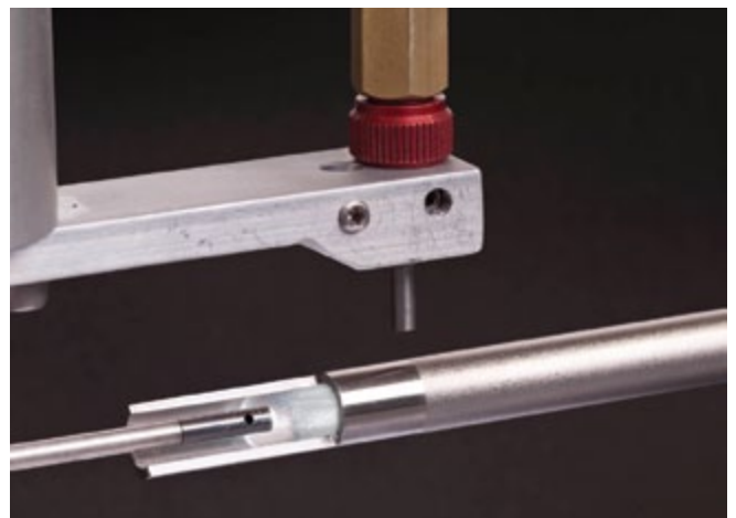
Small ID/OD are peened simultaneously
