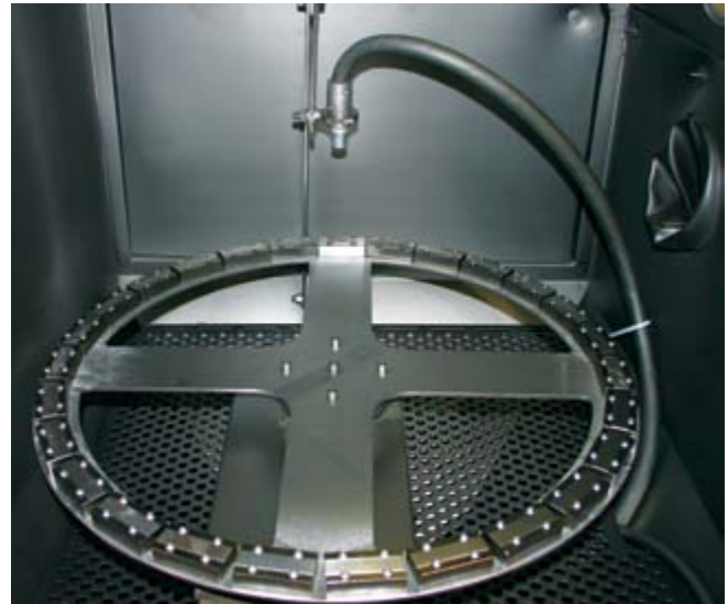
Almen strips are shot peened in a custom air blast cabinet in Electronics Inc.'s test laboratory as part of EI's performance testing program.
