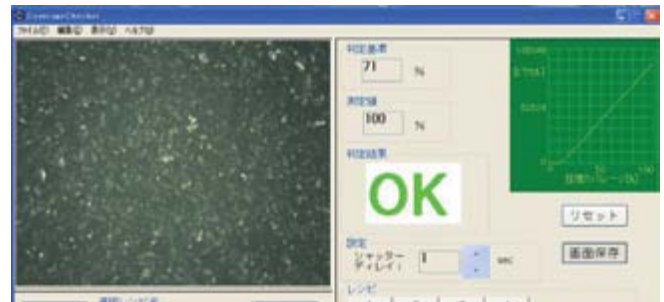
Fig.2 Quantifying blasted area by Coverage Checker™
