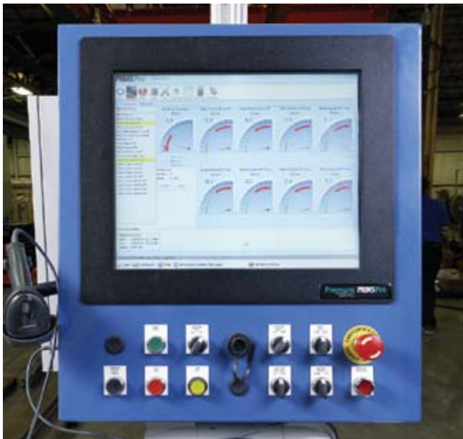
The two-sided CNC-controlled shot peener has the PRIMS Pro Operator Interface for process control, monitoring, PM and report generating
