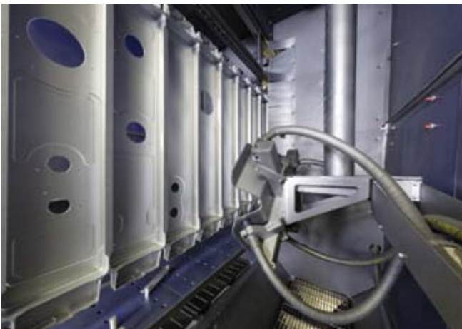
An asymmetrical part with varying thicknesses in the vertical two-sided robotic shot peening machine
