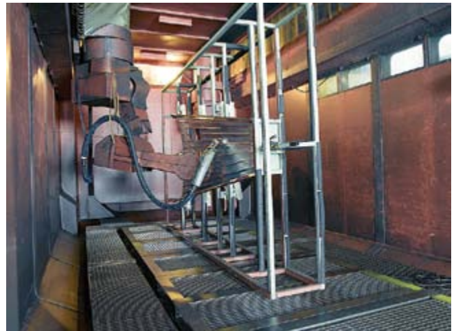
KSA's peen forming processes are fully automated.
